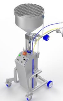
Type: FF500-V1 in vertical single head execution – pneumatically driven with 40L conical hopper. Compact footprint. Application: for filling soups/sauces/mashed potatoes and more
